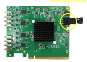
RU1388C relies on two power sources to support eight USB Devices, power supplied through the PCIe bus, and power from the system's PSU via an external 6 pin PCIe power cable. If the external cable is not connected, there will be insufficient power to support all 8 USB Devices; this may cause the USB Device to drop offline.
