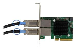
The other end of the SFF-8088 to SFF-8088 connects to the RS6418S SFF-8088 connector as illustrated below (a to a, and b to b), RS6418S connects to SAS/SATA hard drives or SSD's, and connect to AC power;
