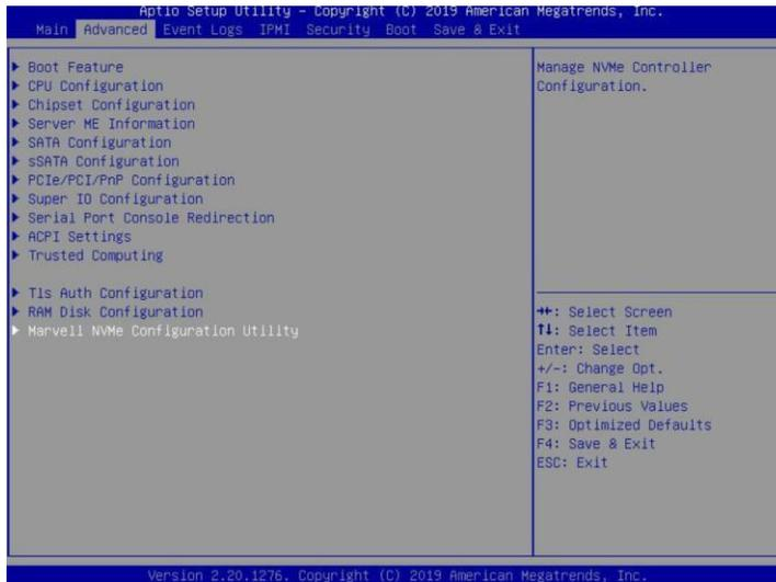
*Note: If you cannot find “**Marvell NVMe Configuration Utility**” in the motherboard BIOS under “**advanced**” interface, you will need to create the array using one of the other four methods.*
