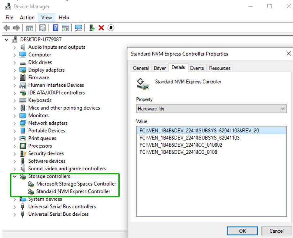
If the interface does not display “Standard NVMe Express Controller”, then the motherboard does not recognize the SSD6200.
