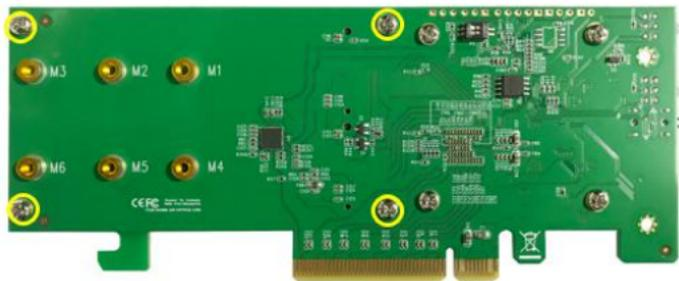
**Note:** Make sure the aluminum cover is properly aligned with the controller board (PCB), and that it makes full contact with the thermal pad, before refastening it to the SS6202. If the cover is improperly installed, thermal pad will be unable to sufficiently cool the NVMe SSD's and controller componentry, which may result in damage to the SSD's or controller hardware, performance loss, unstable I/O, and the loss of data.
