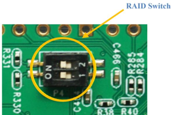
**RAID Switch:** four options are available; when the system starts, the SSD6202 will automatically create the specified array using the hosted NVMe SSD's.
