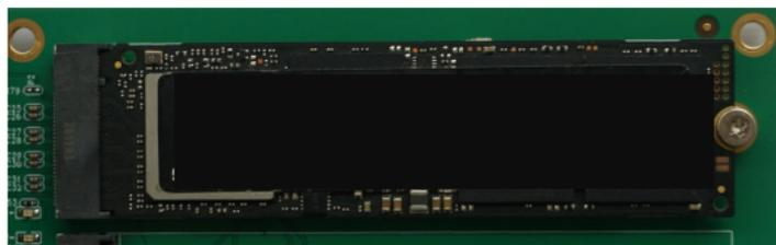
**Note:** Make sure the SSD's are carefully, but securely installed into each M.2 port. Loose connections can cause a variety of stability and performance issues, and may ultimately result in data loss.
