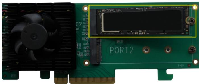
Step 4. Refasten the screw to secure the SSD.
