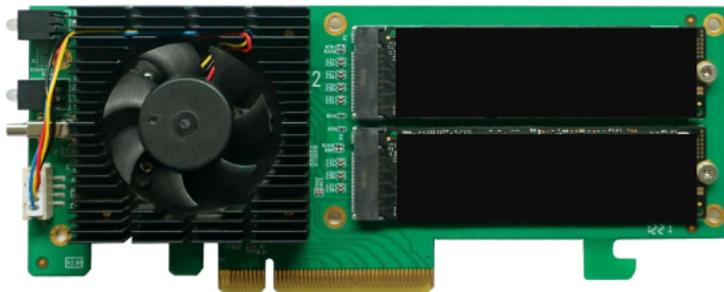
Step 6. Align and install the heatsink; on the rear of the SSD6202, refasten the 4 screws that were removed in step 1.
