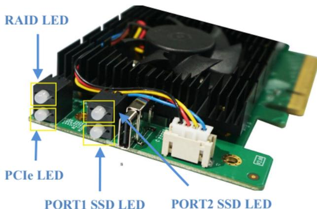
**RAID LED:** when the SSD6202 has no RAID, the RAID LED is off. If there is a normal RAID in the SSD6202, the RAID LED is green. If the RAID is fail (RAID Status is Disable or Critical), the RAID LED is red.
