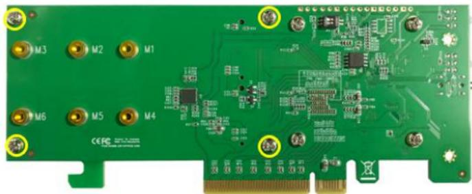
After removing the screws, carefully remove the heat sink from the SSD6202.
