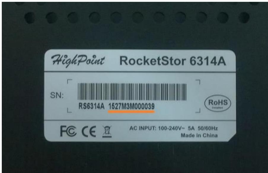
The S/N has 13 characters and the S/N format for the RocketStor 6314X is “\*\*\*\*M3M\*\*\*\*\*”
