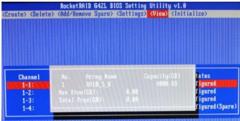
RAID Array – This option will display information about each RAID array hosted by the HBA. Highlight the target device and press Enter to view details about the configuration.
