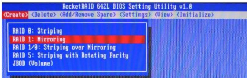
1. Use the arrow keys to select the RAID level and press Enter key.
