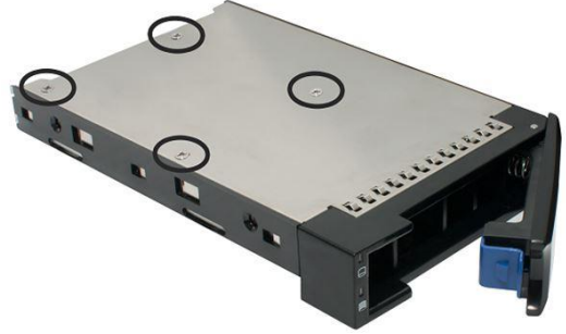
Figure 4. 2.5" SSD Mounting Holes
