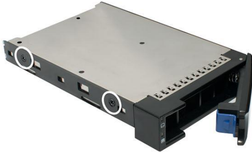
Figure 3. 3.5" HDD Mounting Holes
