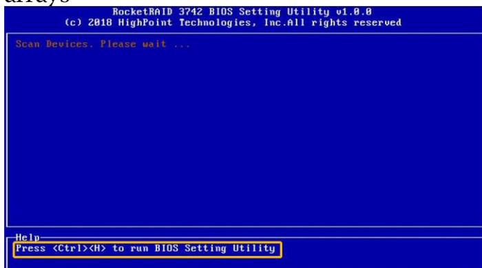
Figure. RocketRAID Splash Screen. Press CTRL + H to enter BIOS
