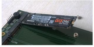
Step 5. Refasten the screw to secure the SSD.
