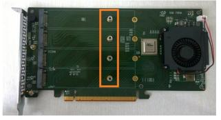
Step 3. The SSDs should be installed from top to bottom. Remove the top screw.
