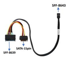
4. Shown above is an SFF-8643 to U.2 SFF-8639 cable with a 15-pin SATA power connector. Connect the SSD7120 to the NVMe SSD's using the appropriate SFF-8643 cables. The SFF-8639 port should be connected to the NVMe SSD's U.2 port. The 15 pin SATA power connector should be connected the system's power supply.
