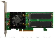
Step 7. Replace the heat sink after installing all SSDsStep 8. On the rear of the SSD7202, refasten the 4 screws that were removed in step 1.
