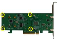
After removing the screws, carefully remove the heat sink from the SSD7202.
