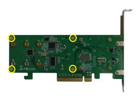
**Note:** Make sure the aluminum cover is properly aligned with the controller board (PCB), and that it makes full contact with the thermal pad, before refastening it to the SSD7202. If the cover is improperly installed, thermal pad will be unable to sufficiently cool the NVMe SSD's and controller componentry, which may result in damage to the SSD's or controller hardware, performance loss, unstable I/O, and the loss of data.
