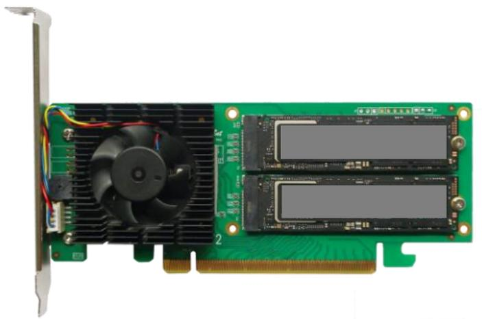
**Note:** Make sure the SSD's are carefully, but securely installed into each M.2 port. Loose connections can cause a variety of stability and performance issues, and may ultimately result in data loss.
