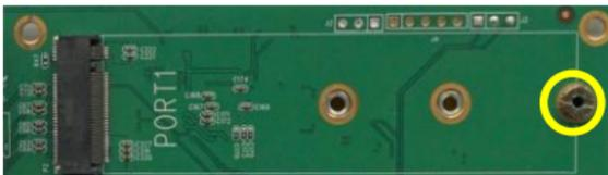
Step 5. Gently insert the SSD into the slot. Refasten the screw to secure the SSD.
