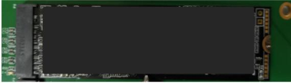
Step 6. Refasten the screw to secure the SSD.
