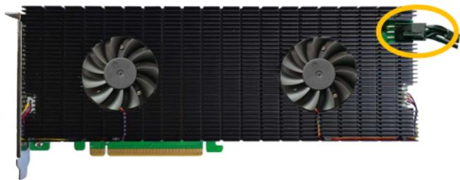
SSD7540 relies on two power sources to support eight SSDs; power supplied through the PCIe bus, and power from the system's PSU via an external 6 pin PCIe power cable. If the external cable is not connected, there will be insufficient power to support all 8 SSD's; this may cause the SSDs to drop offline.
