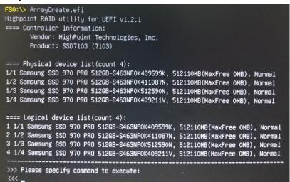
g. Next, create the array using the following command: create RAID0
