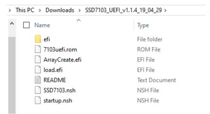
*Note:* If the above content is not present in the root directory, the UEFI boot device will not be properly recognized, and/or you will be unable to create an array for OS installation.
