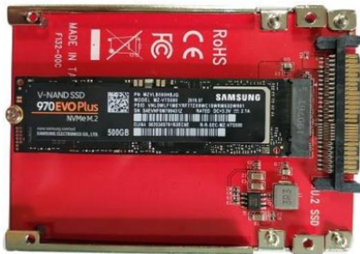
5. Carefully insert the ‘M.2 Drive to U.2 Host Adapter’ into each disk tray and secure them with the provided mounting screws.
