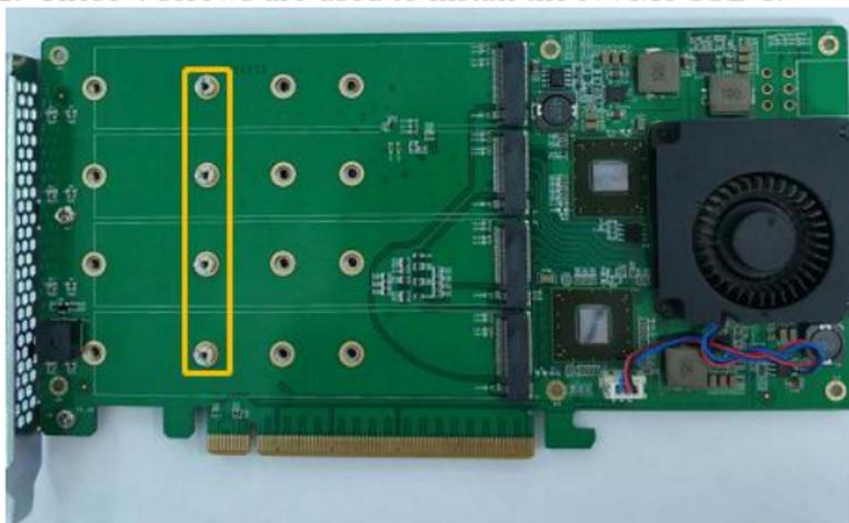
Step 3. The SSDs should be installed from top to bottom. Remove the top screw.
