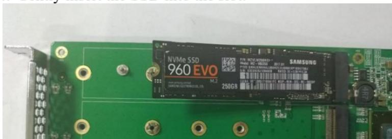
Step 5. Refasten the screw to secure the SSD.
