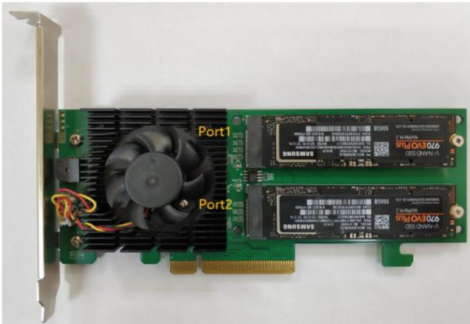
Step 6. Replace the heat sink after installing all SSDs
