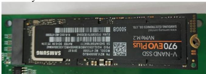
Step 5. Refasten the screw to secure the SSD.
