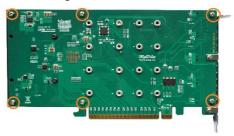
After removing the screws, carefully remove the casing from the R1101.
