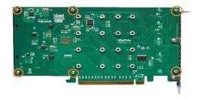
Note: Make sure the aluminum cover is properly aligned with the controller board (PCB), and that it makes full contact with the thermal pad, before refastening it to the R1101. If the cover is improperly installed, the fan and thermal pad will be unable to sufficiently cool the NVMe SSD's and controller componentry, which may result in damage to the SSD's or controller hardware, performance loss, unstable I/O, and the loss of data.
