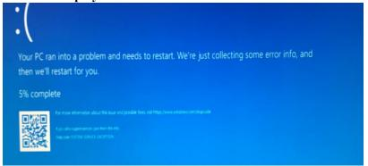
If you are running Windows 10, please make sure that any **Quick Shutdown** options are disabled – these features can cause a BSOD when the SSD7101A-1/SSD7204/SSD7104/SSD7120/SSD6540 /SSD6540M/SSD7180/SSD7184/SSD7140 is installed into or removed from your motherboard. BSODs can be avoided by **completely powering off** your system.
