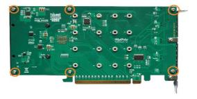
**Note:** Make sure the aluminum cover is properly aligned with the controller board (PCB), and that it makes full contact with the thermal pad, before refastening it to the SSD7101A-1. If the cover is improperly installed, the fan and thermal pad will be unable to
